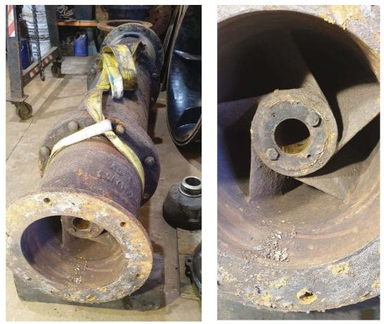
Overhaul of the impeller, impeller housing, replacing bottom bush and top thrust bearings is estimated at  $\pounds$ 11,000.00 + VAT and Perry's are in the process of arranging haulage/lifting to return and re-commission.
