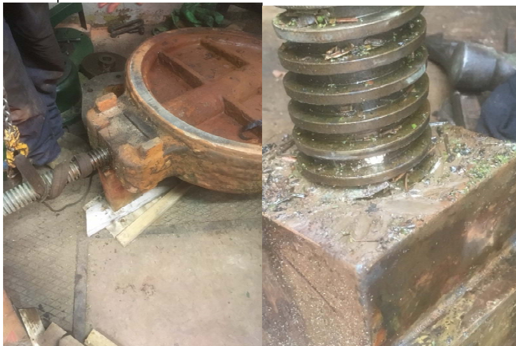
Damage to the threads of the shaft.
