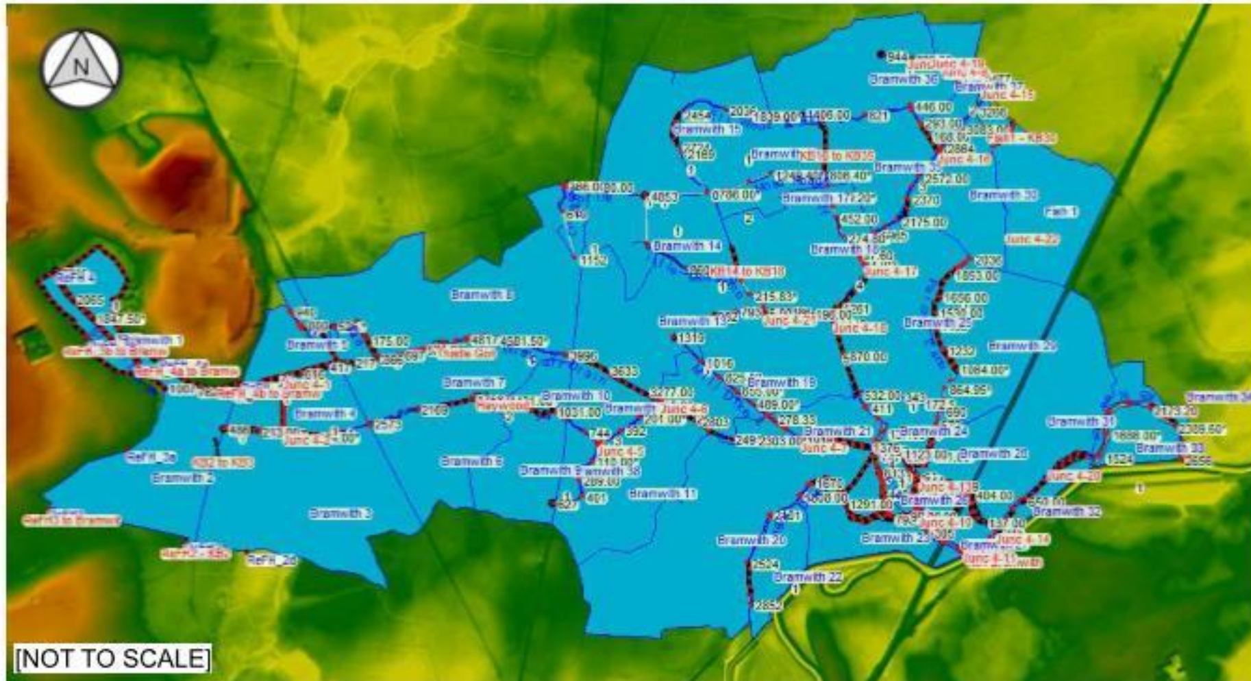
Figure 4-2: Kirk Bramwith HEC-RAS model schematic view
